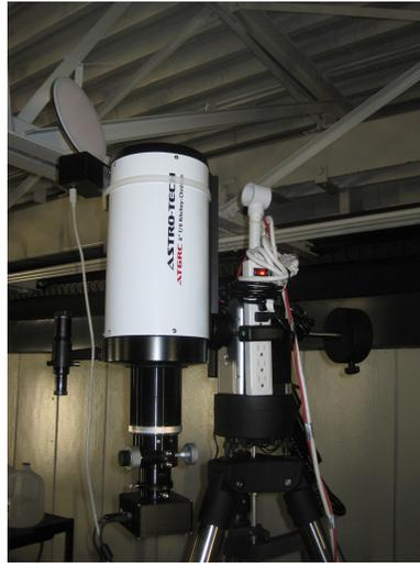
**Figure 3.4** The replacement wide-field f/9 Ritchey-Chrétien telescope on the robotic mount, shown with the cord wrap prevention rod mounted in its temporary housing at the Rankin Science Observatory.
