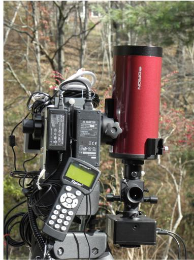
**Figure 3.3** The original Orion telescope on the robotic mount, shown without the cord wrap prevention rod mounted.
